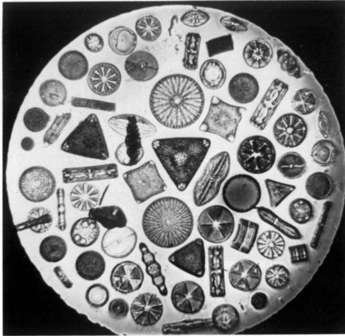
Fig. 17(a). Photograph taken through a lens made in the style of Leeuwenhoek, giving a measured resolving power of 2.5 \mu\text{m} .
