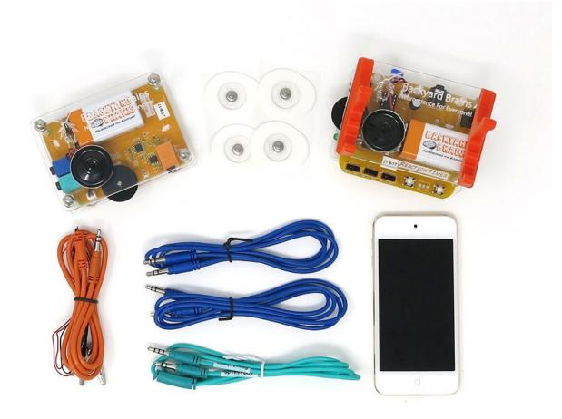
2. For PC Users: Use two laptop cables (blue) to connect your Reaction Timer to the Muscle SpikerBox and to your Computer. The first blue Laptop Cable connects from your Muscle SpikerBox to your Reaction Timer's "SpikerBox" port. The second blue Laptop Cable connects your computer's microphone input to the port labeled "Smartphone...." Yea, just trust us. Plug it into the SmartPhone port even when you're using a computer!
