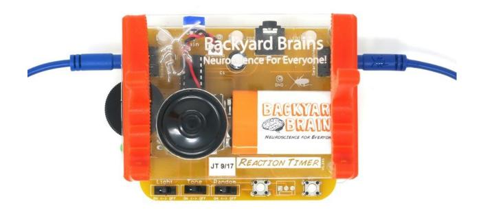
3. For Mac or Smartphone/Tablet users: Use a laptop cable (blue) to connect the Muscle SpikerBox to the Reaction Timer's "SpikerBox" port.
